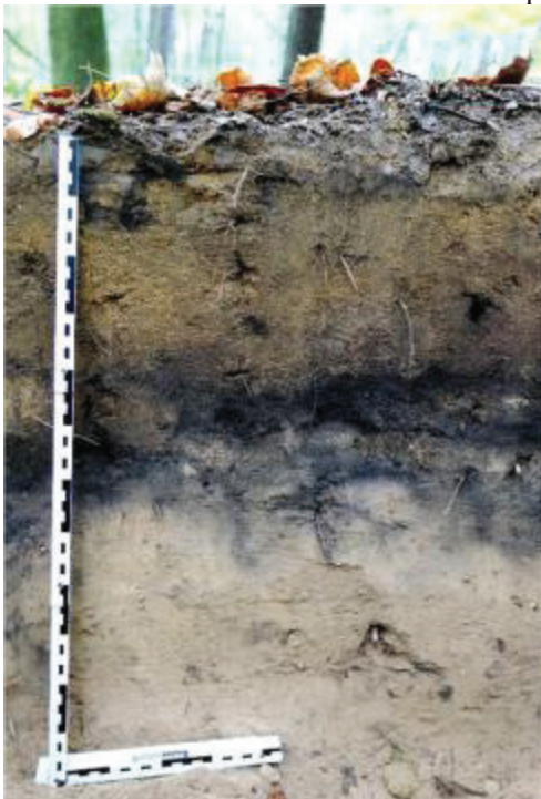
Fig. 1: Regosol developed at the edge of a bomb crater over 75 years on a layer of a thickness of about 25 cm ejected soil material overlying the buried original top soil (Podzol - Duisburg/Germany).
